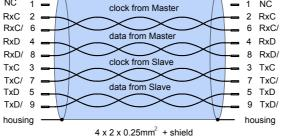
SSK14 must not be used on a COMPAX which is configured as a master (P243=1).
